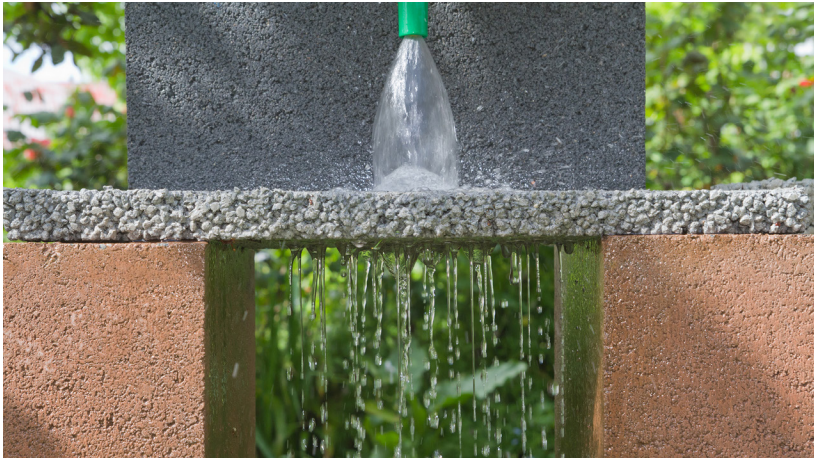
Permeable paving reduces stormwater runoff and recharges groundwater
